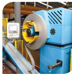
The material can be cut at different dimensions, at various widths and lengths. GOS lamination requires a high degree of precision. Therefore, we routinely perform strong quality checks which measure burr level, stack height, weight and other dimensions.
